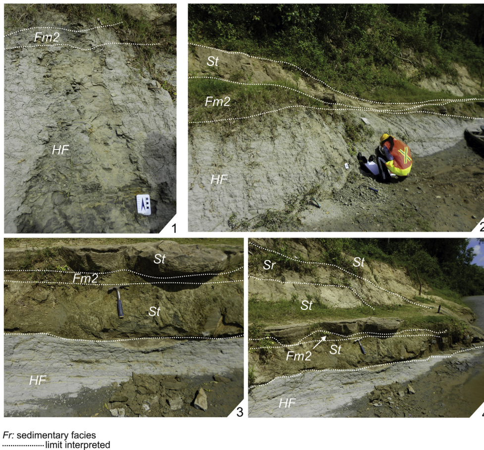
Fig. 6. Sedimentary facies identified in the Querru 1 outcrop, Itapecuru Formation. 1. Facies HF, mudstone with linsen and subordinately wavy lamination, intensely bioturbated. Facies Fm2, massive silty mudstone, light olive-grey. 2. Facies St, medium sandstone with small-scale trough cross stratification. 3. Facies St, medium sandstone with trough cross stratification. 4. General aspect of the outcrop.
