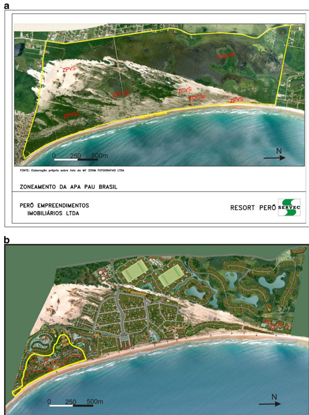
Fig. 3 a Pau Brasil Environmental Protection Area (APA) zoning plan in the dune field area; yellow line represents the resort's limits. ZCVS Wildlife conservation zone, ZPVS wildlife preservation zone (both referring to mobile dunes), ZOC controlled occupation zones (stationary dunes and adjacent wetland areas). b Resort's master plan. Note the total occupation of the fixed dunes and of the adjacent wetland area; yellow line indicates the area of Club Med already licensed for construction. Image source: Project's Environmental Impact Study (modified from SERVEC 2007)
